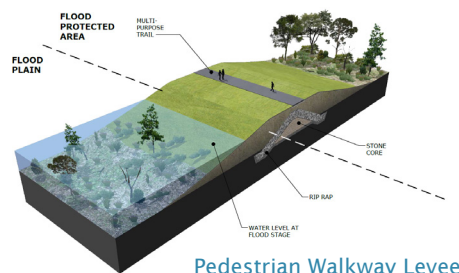
Pedestrian Walkway Levee
