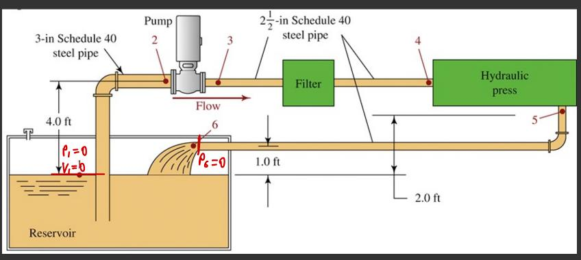
$$\frac{V_2^2}{2g} + \frac{P_1}{p} + Z_2 = \frac{V_1^2}{2g} + \frac{P_1}{p} + Z_1 + h_{R+1}$$
