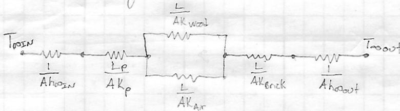
$$R_{\infty \text{in}} = \frac{1}{Ah_{\infty \text{in}}} = \frac{1}{(1.33 \text{ ft}^2)(3 \text{ BTU/hr} \cdot \text{ft}^2 \cdot \text{R})} = 0.2506 \frac{\text{hr} \cdot \text{R}}{\text{BTU}}$$
