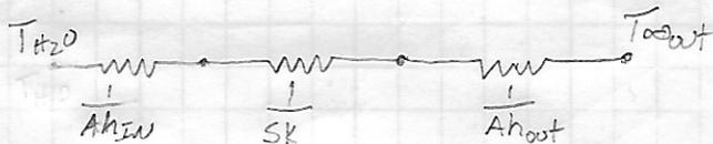
$$R_{IN} = \frac{1}{A h_{TW}} = \frac{1}{(1\text{m})^2(1189.36 \text{ W/m}^2\text{}\cdot\text{C})} = .000841 \text{ W/C}$$
