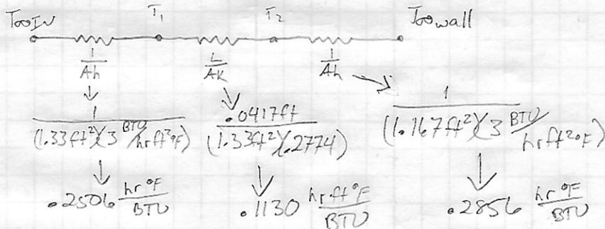
$$Q = \frac{T_{0,air} - T_{0,wall}}{R_{eq}}$$
