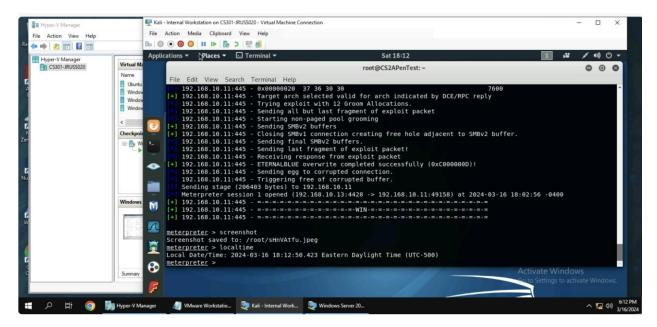
(In the above screenshot, the localtime command is used to determine the date and time of the remote host)
