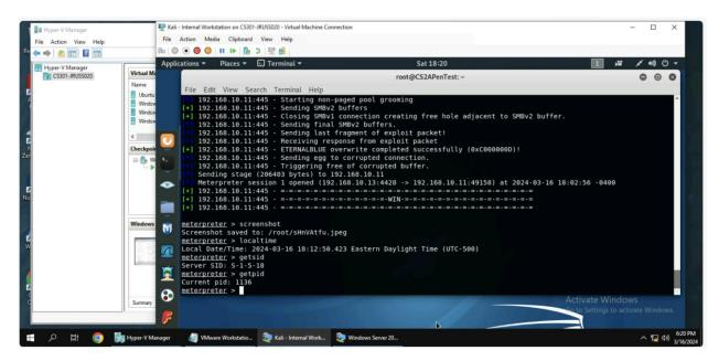
(In the above screenshot, the getpid command is used to get the process id of the target machine)
