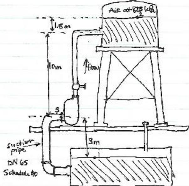
$$h_A + \frac{P_1}{\gamma} + \frac{V_1^2}{2g} + z_1 = \frac{P_2}{\gamma} + \frac{V_2^2}{2g} + z_2 + h_{L1-2}$$
