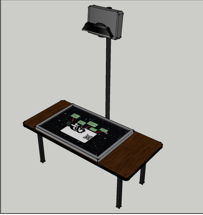
Fig. 2. The conceptual design of the hardware setup of the Tangible Table Top is depicted. The Kinect device and the projector are arranged in a vertical orientation looking downward towards a surface.
