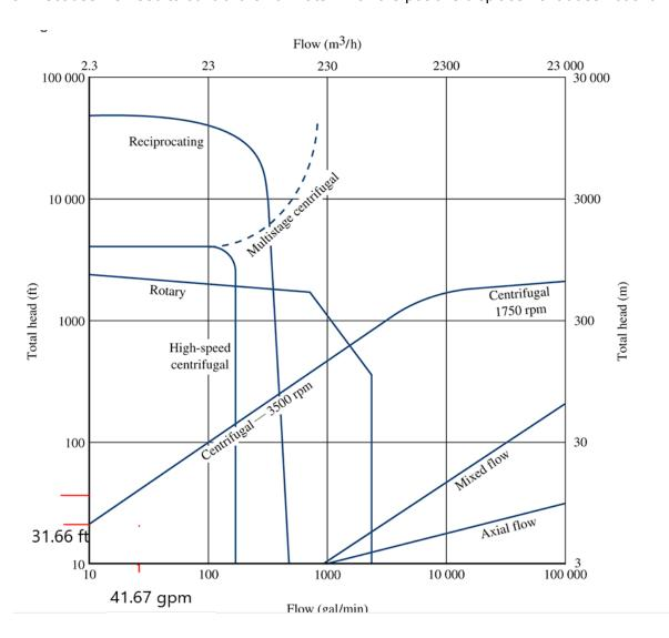
**6.** The size pump we chose was 1x2x7.5 which runs at 3500 rpm and 60 hertz (page 368), the point of operation is specified on the graph in red. (Our pump runs at 1775 rpm)
