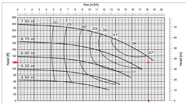
**7.** Based on the power curve we determined that 8.25 BHP is necessary to power the pump properly.
