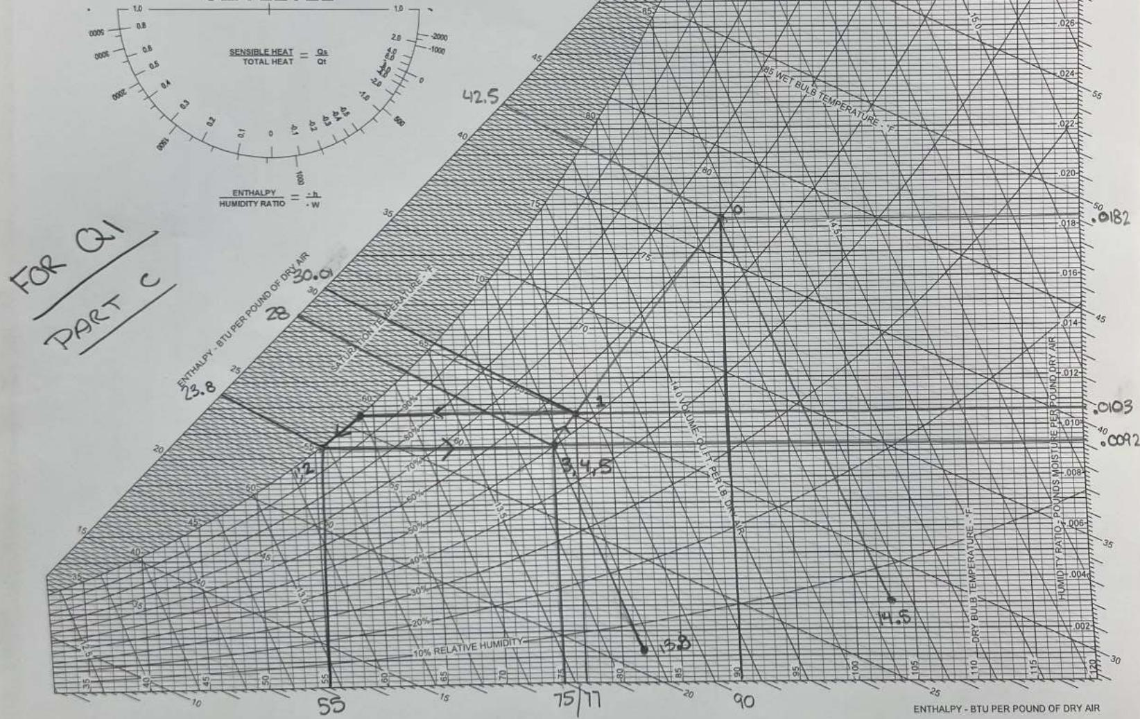
Summary → for this problem we showed that we understood cooling and dehumidifying system. we were able to use the charts and equations in order to find the quantity of air supply, the states at each point, the required capacity, of the cooling and dehumidifying unit. with that being said in order to find the correct values you must correctly do the chart.
