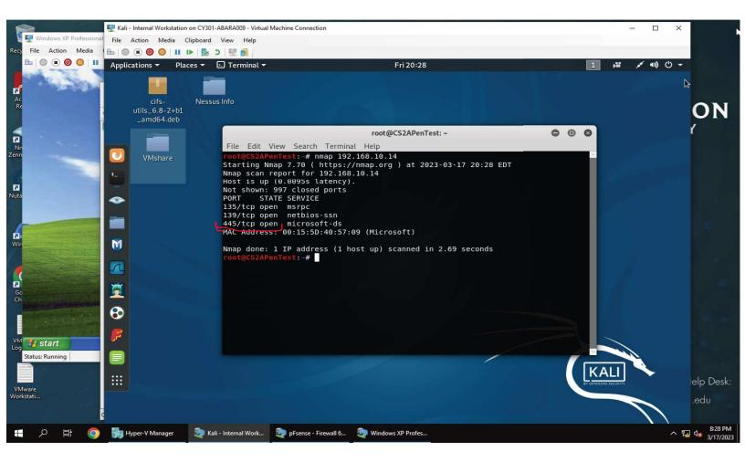
Here, I ran a port scan of Windows XP, using "nmap" command and its IP address of 192.168.10.14. From the scan, the open ports are 135/tcp that uses service msrpc, 139/tcp using service netbios-ssn and port 445/tcp using service msicrosoft-ds. The highlighted port number confirms port 445 is open.
