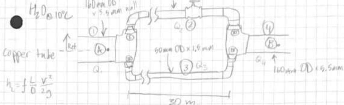
$$\textcircled{2} \frac{\Delta P}{\gamma} = h_{L_{A \rightarrow B_2}} = h_{L_{red II}} + 2h_{L_{elb}} + 2h_{L_{tee}} + h_{L_{valve}} + h_{L_{exp III}} + h_{L_2}$$
