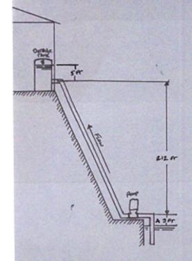
GIVEN!  $P_{g} = 30 \frac{16}{10^{2}} \frac{1000}{100} = 62.4 \frac{16}{100}$   $Q = 40 \frac{600}{1000} \cdot \frac{167^{3}}{14160} \frac{1000}{10000} = 0.089117 \frac{67}{560}$   $P = \frac{P_{g}}{100} = \frac{7000}{74}$ SOLUTION:  $h_{A} + \frac{P_{g}}{N_{c}} + \frac{V_{g}}{V_{g}} + \frac{V_{g}}{V$
