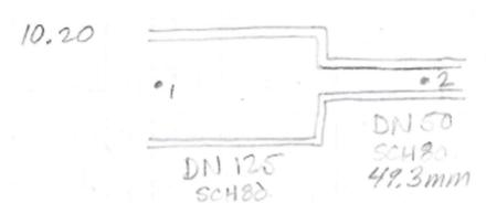
$$h_{z} = K \frac{v^{2}}{2g} \frac{TABLE 10.3A}{FIND K} NEED RATTO D_{1}:D_{2} \frac{122.3 \text{ mm}}{49.3 \text{ mm}} = 2.48$$
