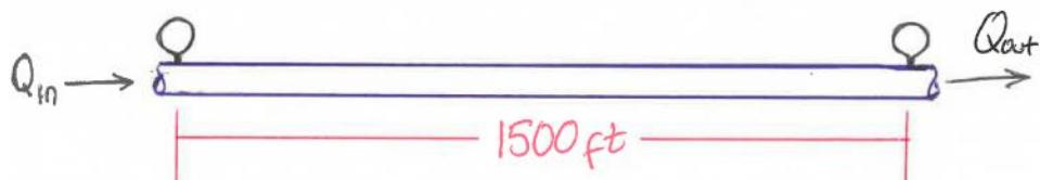
The pipe is modified by adding a loop made of 1 ½ inches standard steel tubing that is only 900 ft long. What is the expected increase in flow rate through the system for the same pressure as in the original pipe (the one you calculated)? Consider all minor losses.
