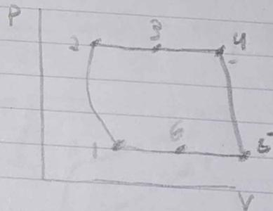
$P_1 = 100 \text{ kPa}$      $T_1 = 303 \text{ K}$      $\frac{T_2}{T_1} = \frac{P_2}{P_1} \frac{1}{r_p}$      $T_2 = 303(10)^{1.4} = 585 \text{ K}$
