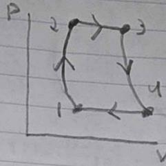
$r_p = \frac{P_2}{P_1} = 10$      $Q_{in} = 500$      $\dot{m} = 1 \text{ kg/s}$      $P_1 = 70 \text{ kPa}$      $T_1 = 0^\circ\text{C} + 273 = 273 \text{ K}$
