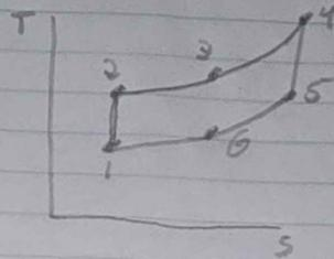
$P_1 = 100 \text{ kPa}$ ,  $T_1 = 300 \text{ K}$ ,  $h_1 = 310.24$ ,  $P_{r1} = 1.555$
