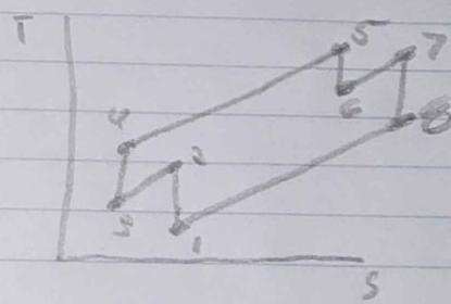
$P_2 = (P_r) P_1 = 3(1.386) = 4.158$ ,  $h_2 = 411.3$ ,  $T_2 = T_4 = 410 \text{ K}$
