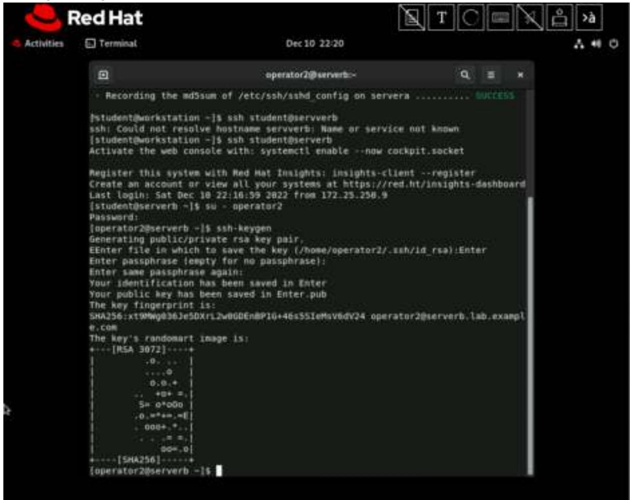
4. Use the `ssh-copy-id` command to send the public key of the SSH key pair to the `operator2` user on the `servera` machine. Use `redhat` as the password for the `operator2` user on `servera`.
