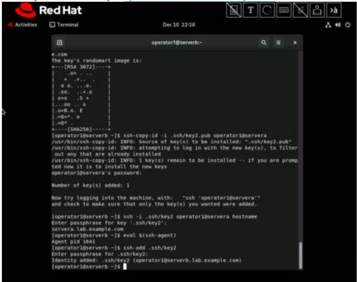
11. Execute the `hostname` command on the `servera` machine remotely without accessing a remote interactive shell. Use the `/home/operator1/.ssh/key2` key as the identity file.
