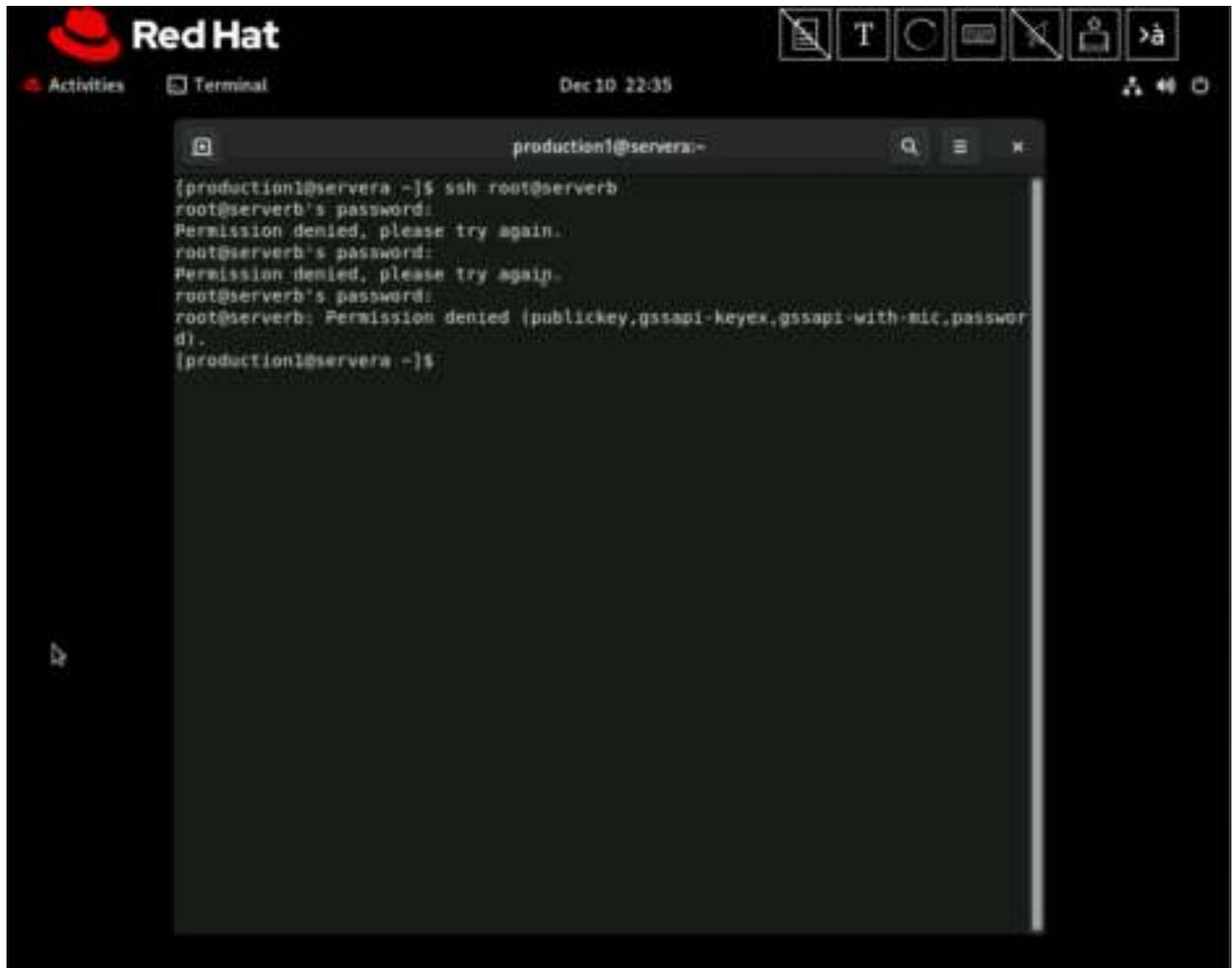
7. Configure the `sshd` service on the `serverb` machine to allow users to authenticate with SSH keys only, rather than with their passwords.
