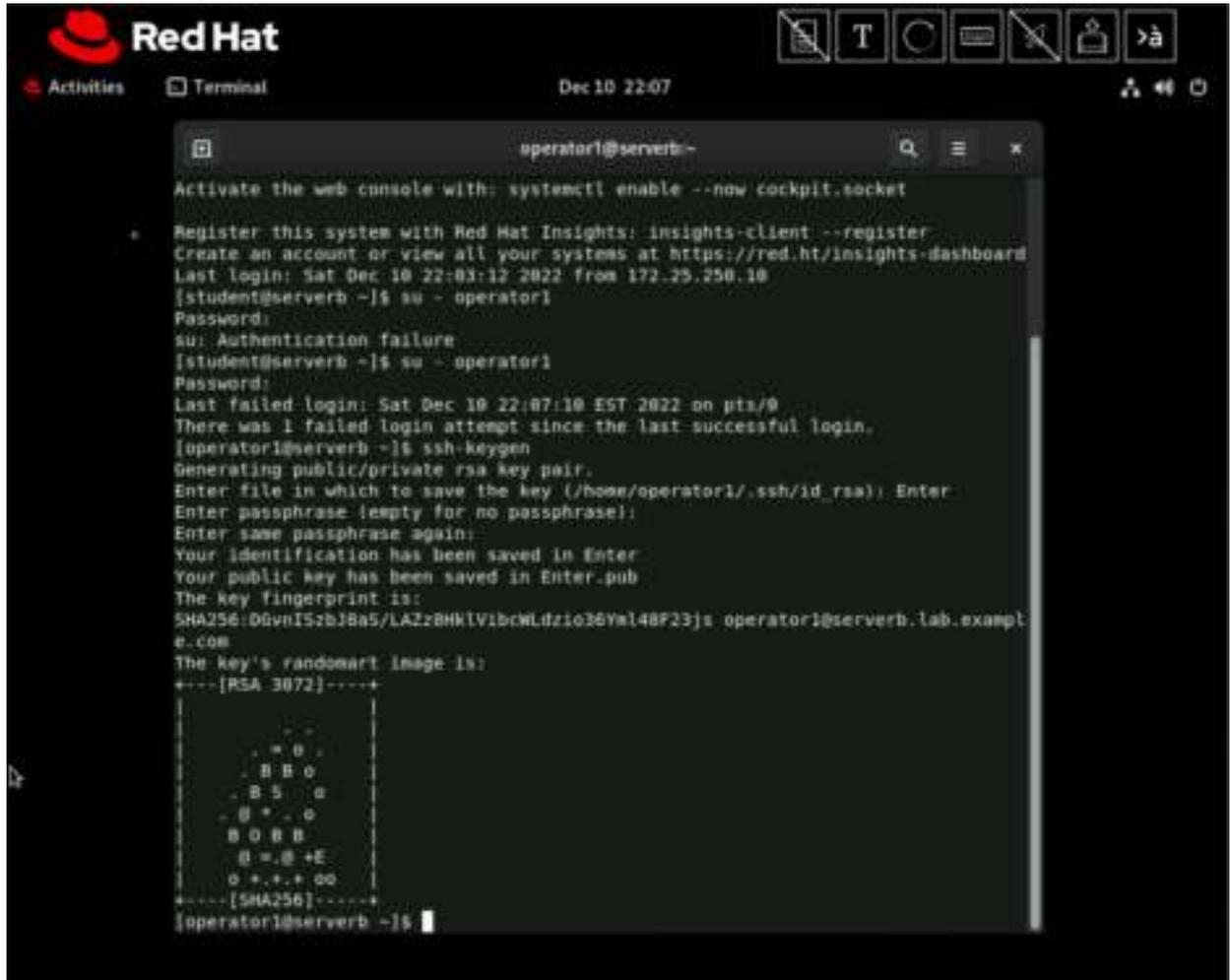
4. Send the public key of the SSH key pair to the operator1 user on the servera machine, with redhat as the password.
