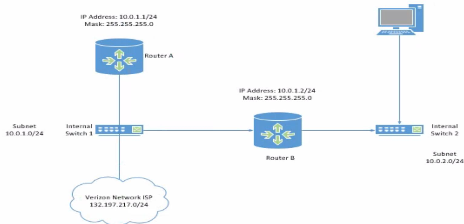
System Routing Table Router A
