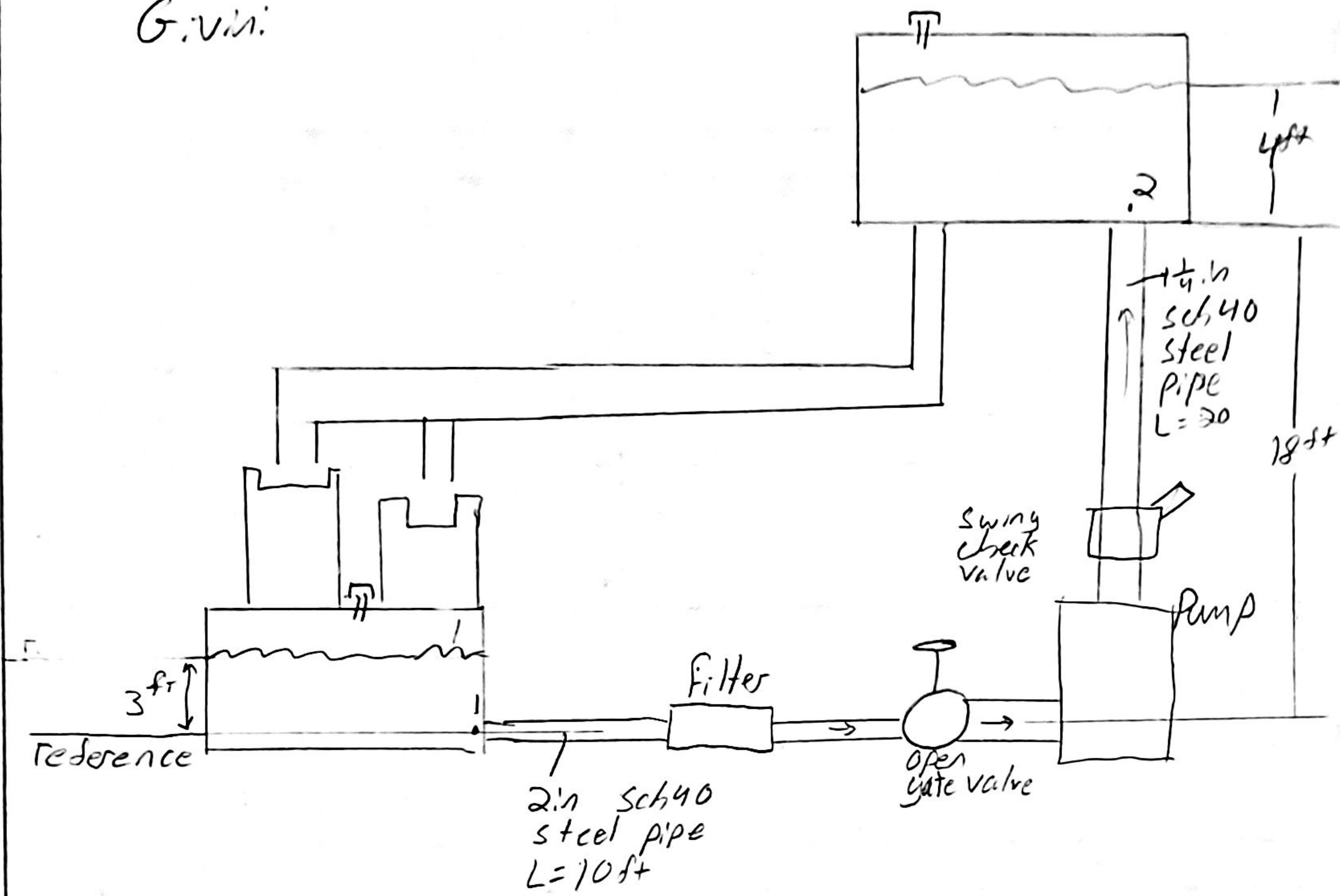
Find: total pump head and power delivered to the coolant
