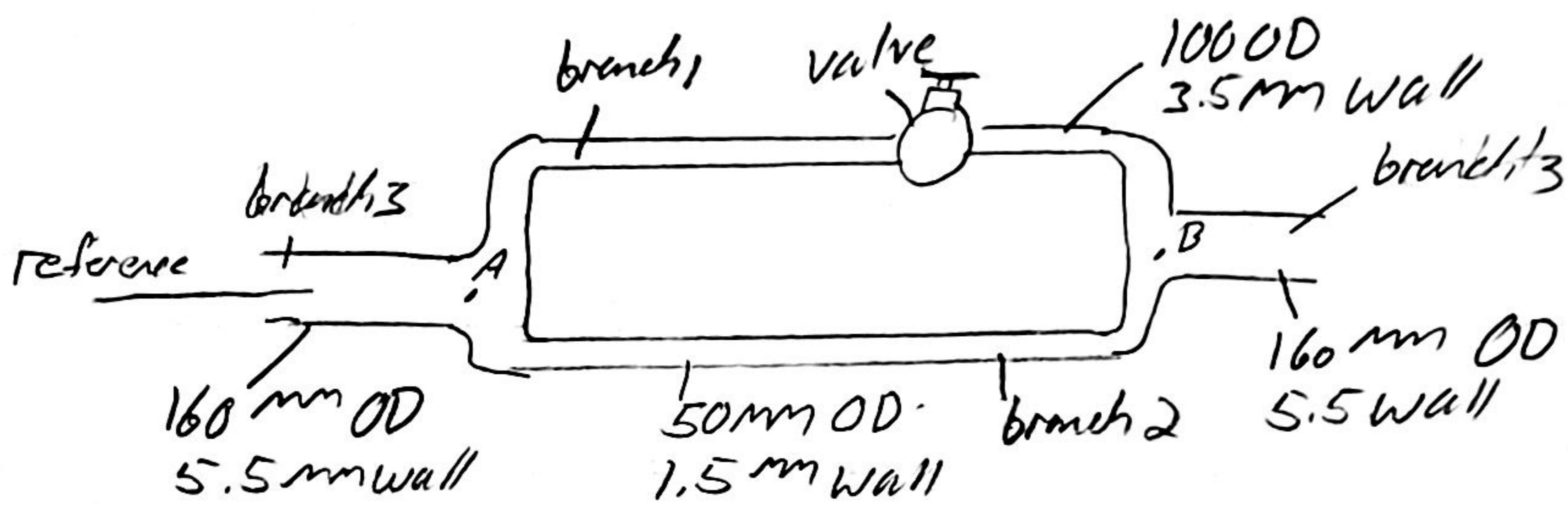
Find: what is the resistance coefficient  $k$  of the valve so that both branches have  $500 \frac{\text{L}}{\text{min}}$  flow rate
