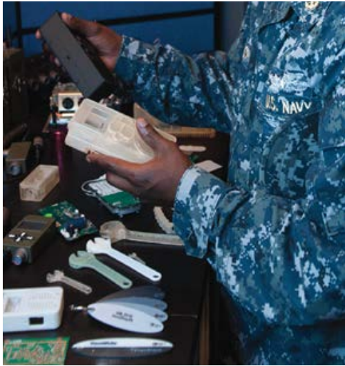
Figure 1: 3D printed maintenance spare parts - wrenches at Print the Fleet workshop at the Navy [1]
