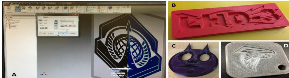
Figure 2: Examples of designs. A: Reverse engineering of a sketch used for extrusion from an image in Autodesk Inventor; B – D: Different designs after 3D printing (Workshop # 1).
