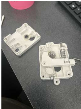
Figure B1. A disassembled material feeder from an older model MakerBot Ultimaker.
