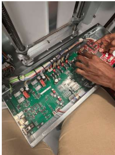
Figure B2. An open side panel of a Trotec Speedy300 laser engraving machine showing the many wires and processors inside.
