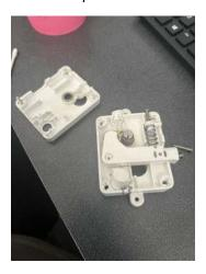
This is an older model 3d printer that I was working with to decide if they can be used for a project. The two main issues were plate adhesion and material feeding malfunctions.
