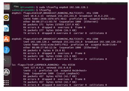
4. Configure the temporary IP address, routing table, and DNS server on Client VM as shown in:
