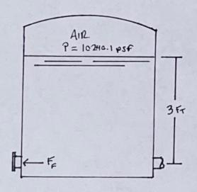
TO SOLVE FOR FORLE ACTING ON BLIND FLANGE ON LEFT-HAND SIDE OF TANK, I WILL START BY SOLVING FOR EQUILIENT DEPTH OF FLUID USING EQUATION FOR PLEZOMETRIC HEAD, ha:
