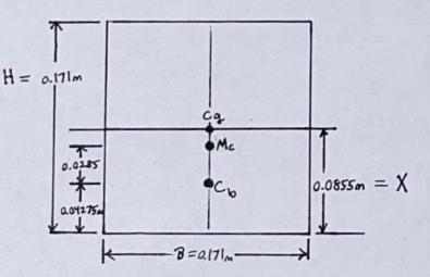
BECAUSE THE CENTER OF GRAVITY APPEARS TO BE ABOVE THE CENTER OF BOUYANCY, I MUST LOCATE THE METACENTER OF THE LOG TO DETERMINE ITS STABILITY IN THE CHANNEL:
