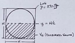
IN axDOOL FOR THE LOG TO FLOAT, THE BOUYANCY FORCE ACTING ON THE LOG MUST BE EQUAL TO THE WEIGHT OF THE LOG. THE FOLLOWING EQUATIONS CAN Bé USED:
