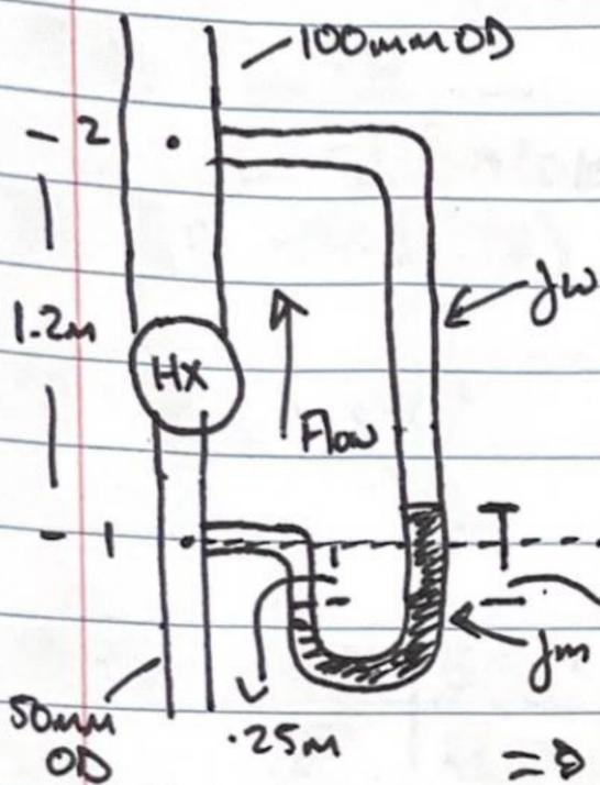
$$v_1 = Q/A_1 = \frac{.006 \text{ m}^3/\text{s}}{1.662 \times 10^{-3} \text{ m}^2} = 3.61 \text{ m/s}$$
