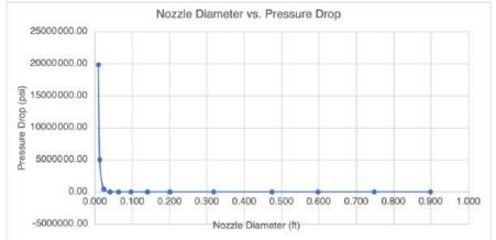
Analysis: The results make sense, as explained in the analysis part of part A, the addition of a nozzle makes the area of flow smaller, making then the power of the pump higher than the system without the nozzle. And the biggle the diameter the nozzle the smaller the pressure drop through that nozzle is
