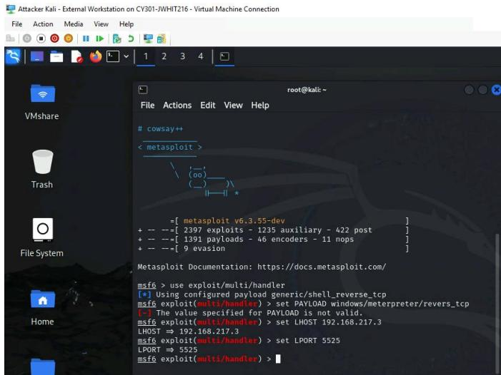
By using the command “msfconsole” lauching the Metasploit program I used the command “use exploit/mulit/handler” to set a name for the exploit and set the payload, host of the payload, and the port in which it will process through.
