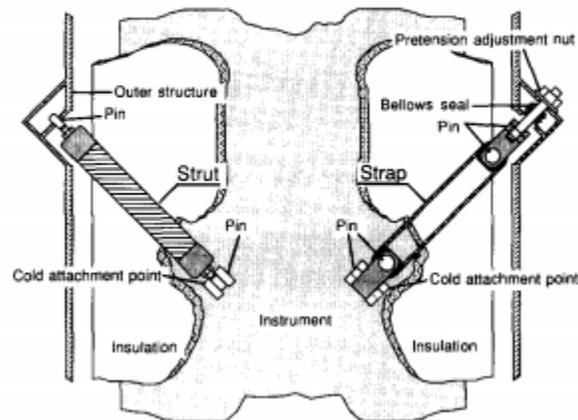
*Figure 2-1 A Schematic of Strut Vs Strap Supports [8]*
