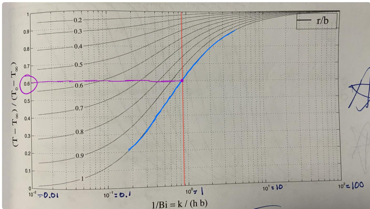
$$\frac{T - T_{\infty}}{T_0 - T_{\infty}} = 0.6 \quad \therefore T = (0.6)(T_0 - T_{\infty}) + T_{\infty} = (0.6)(5^\circ\text{C}) + (25^\circ\text{C})$$
