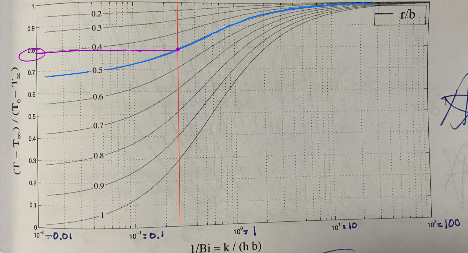
$$\therefore \frac{T - T_{\infty}}{T_0 - T_{\infty}} = 0.95 \Rightarrow T = (0.95)(T_0 - T_{\infty}) + T_{\infty} = (0.95)(5^{\circ}\text{C}) + 25^{\circ}\text{C}$$
