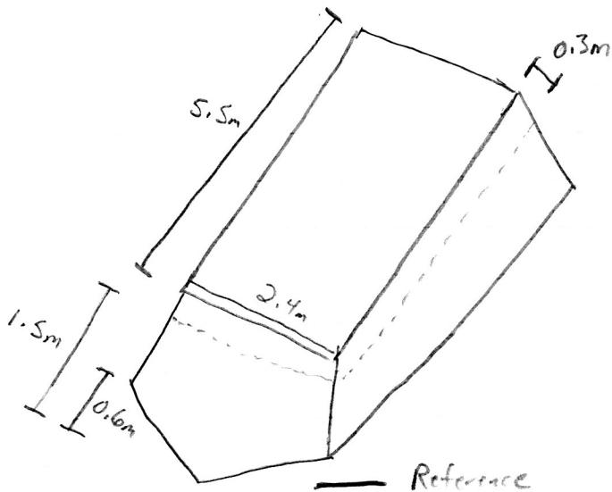
We know that a floating body is stable if the center of gravity is below the metacenter.
