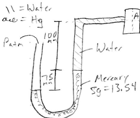
Solution:  $P_A + \gamma_w \cdot h_w + \gamma_{Hg} \cdot h_{Hg} = P_{atm}$
