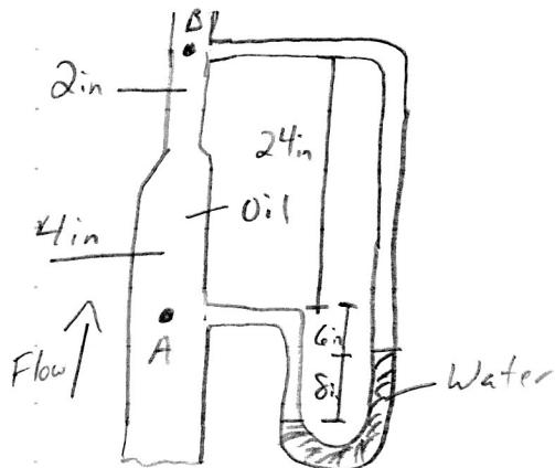
$$\begin{aligned} \text{We know } A_A V_A &= A_B V_B \\ \rightarrow \left(\frac{\pi(4\text{in})^2}{4}\right) V_A &= \left(\frac{\pi(2\text{in})^2}{4}\right) V_B \\ \rightarrow V_B &= 4V_A \end{aligned}$$
