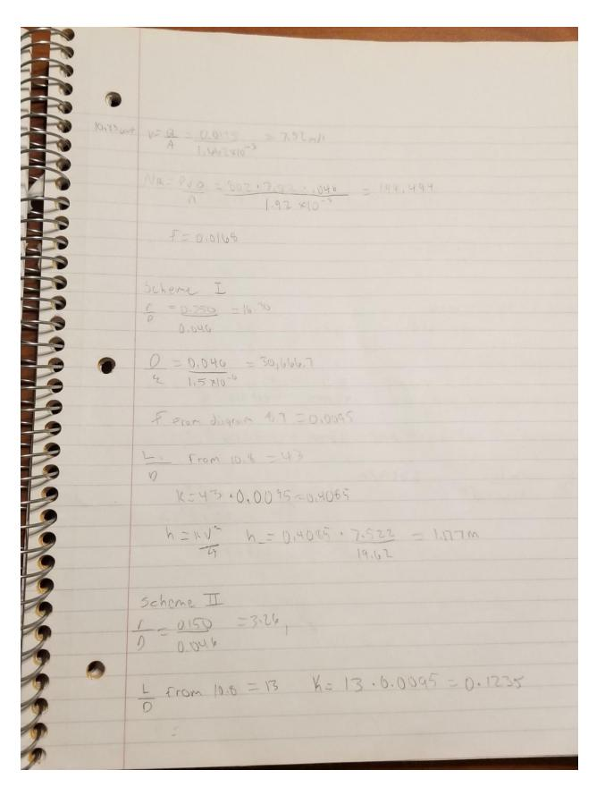
10,48 0=27.5 sulmin -0.0413 FF7/5 0.090) Ft - 1.054 10 6.41×10-3 V= Q = 0.0013 = 9.564+15 0 = 0.0903 = 602 from Diagran \$ = 0.0225 K=(L) FH 5 K = 13,0.0225 = 0.2425 h\_= KV2 = h\_ = 0.2925. 7.522 = 0.415 ft
