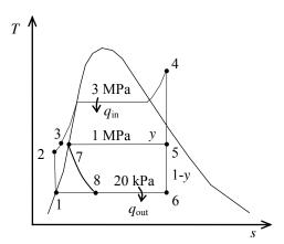
10-53 A steam power plant operates on an ideal regenerative Rankine cycle with two feedwater heaters, one closed and one open. The mass flow rate of steam through the boiler for a net power output of 400 MW and the thermal efficiency of the cycle are to be determined.
