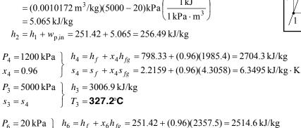
$$\begin{array}{l} P_6 = 20 \, \mathrm{kPa} \\ x_6 = 0.96 \end{array} \} \begin{array}{l} h_6 = h_f \, + x_6 h_{fg} = 251.42 + (0.96)(2357.5) = 2514.6 \, \mathrm{kJ/kg} \\ x_6 = 0.96 \end{array} \} \begin{array}{l} s_6 = s_f \, + x_6 s_{fg} = 0.8320 + (0.96)(7.0752) = 7.6242 \, \mathrm{kJ/kg \cdot K} \\ P_5 = 1200 \, \mathrm{kPa} \\ s_5 = s_6 \end{array} \} \begin{array}{l} h_5 = 3436.0 \, \mathrm{kJ/kg} \\ T_5 = \mathbf{481.1^{\circ}C} \end{array}$$
