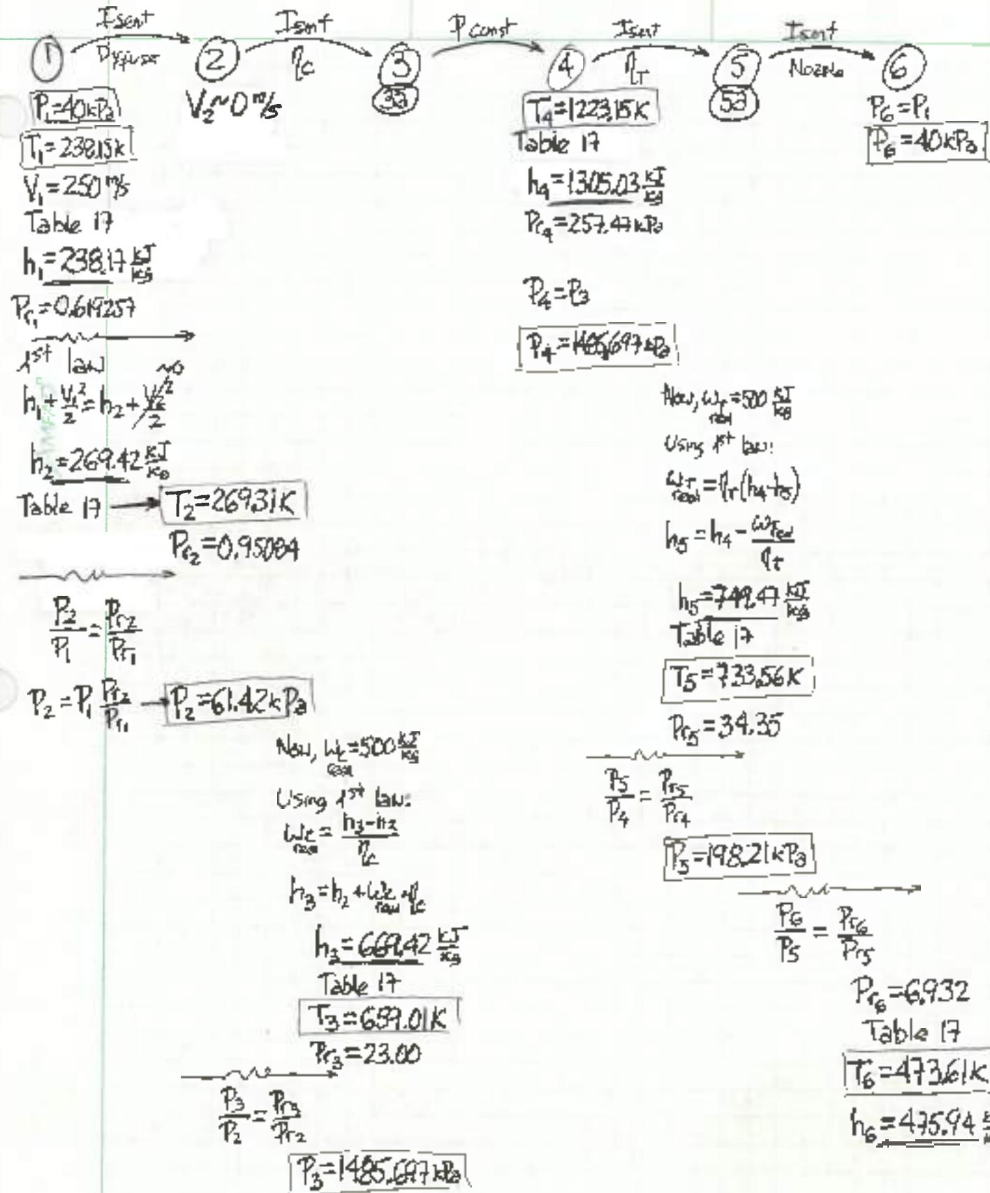
The actual conditions at compressor and turbine exit are:
