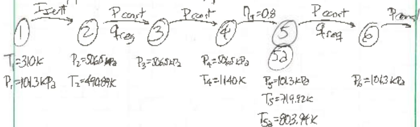
$$\epsilon = \frac{T_3 - T_2}{T_{5a} - T_2}$$
