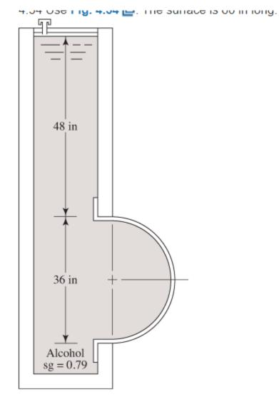
54 D= 36in Sg=0.79 ww=60in hi= 48in Area to of semi circle A= TD2 A=508.9 102 Volume V=AW V= 30535.8123 = 17.67473 weisher of alcohol Ya= 62.4 . 59 Ya= 49.29 16/47 VOIUNE WEISHT  $Wv = V \cdot Ya$ Wu= 87/16 Vertilete porce company Fv=871 1b
