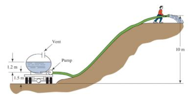
8-38  $\frac{P_{1}}{Y} + Z_{1} + \frac{V_{1}^{2}}{29} + hA = \frac{P_{2}}{Y} + Z_{2} + \frac{V_{1}^{2}}{29} + hL$   $hA = \frac{P_{2}}{Y} - \frac{P_{2}}{Y} + Z_{2} - Z_{1} + \frac{V_{2}^{2}}{29} + hL$   $A = \frac{\pi d^{2}}{4}$  d = 0.025 mA=4.909×10-42 V= A Q=1.583.103 m/s V=3,22n/5 P= 59.P P=1100 K9/ms RE= Pud n= 2 > 103 Re= 44275 F=0.024 h=f=xV2 L=85m hL= 43.122m
