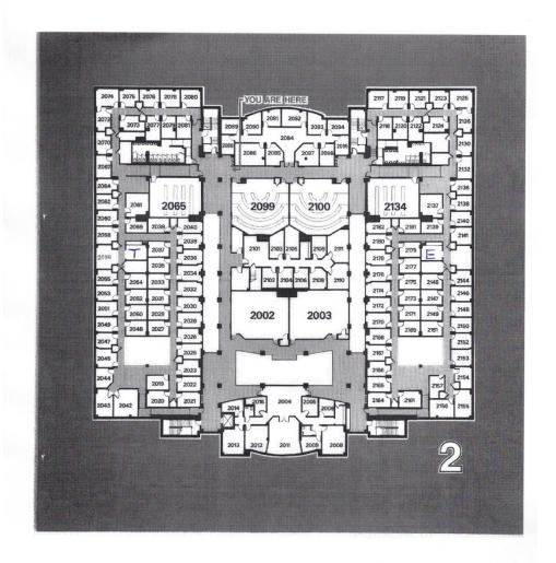
2. An estimate of the total amount of cable that will be needed. The simplest way to estimate is to average the shortest and longest cable runs to each equipment room and telecom closet, then multiply that by the number of cables running to that room. Show the assumptions that you used about the horizontal and vertical cable runs that led you to that number (i.e., show your work).
