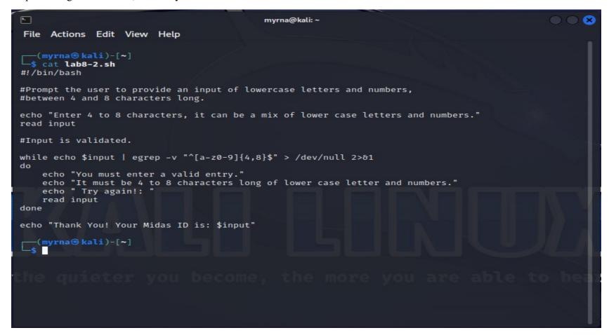
Step 4: We test the program 4 times. First test we added an uppercase letter and the program correctly ask for a valid entry. The second test we added less than 4 digits, again the program asked for a valid entry. The third test we added more than 8 characters and the program one more time asked for a valid entry. Finally, we enter the correct number of characters with corresponding types and the program gave us a correct output.
