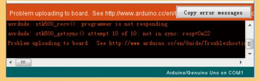
It means that your board is not connected at all, or the drivers have not been installed (if necessary) or that the wrong serial port is selected. If you encounter this, go back to Lesson 3 and check your installation. Once the upload has completed, the board should restart and start blinking.
