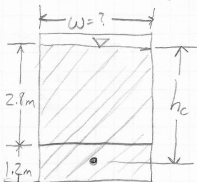
Calculations: Since we already have the force in the vertical direction we can use that to find the unknown dimension for the width.
