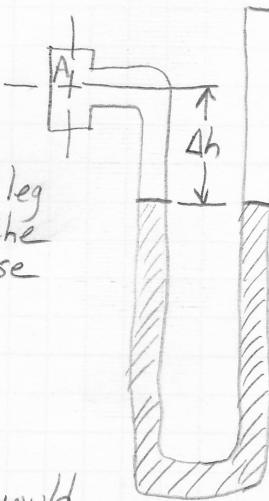
Initial distance from point A to Mercury/water interface was 0.6m
