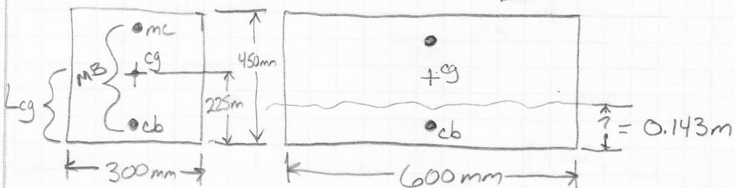
PROCEDURE: we know the distance to center of gravity and the width and length of the package. we can use this data to calculate the center of buoyancy and MB.
