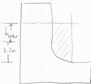
$$27 \text{ KN} = 9.81 \frac{\text{KN}}{\text{m}^3} * \left[ (h_{\text{new}} + 1.2) * 1.2 \text{ m} - \frac{\pi * 1.2^2}{4} \right] * 1.5 \text{ m}$$
