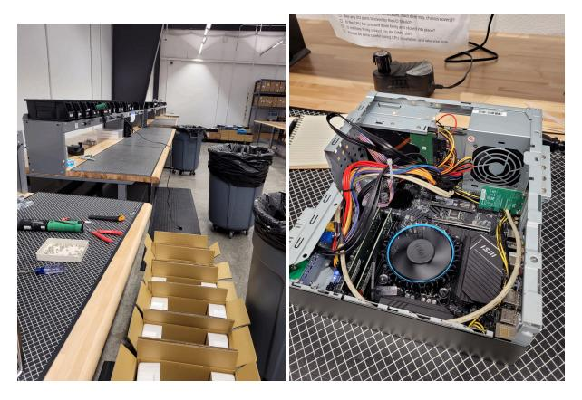
The picture on the left is what the workstations look like where we build the servers. The picture on the right is what a server looks like while we're testing it to make sure it works properly.
